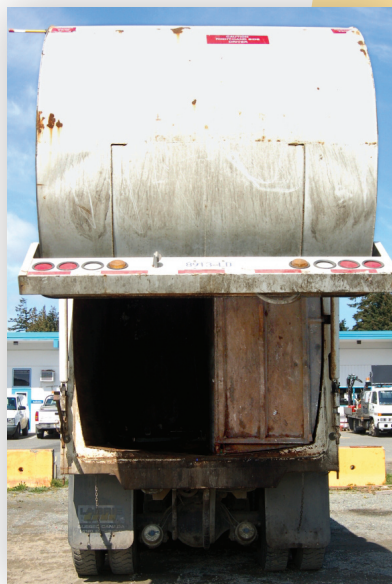
A baffle separates food waste and garbage when they are collected using a single truck.
